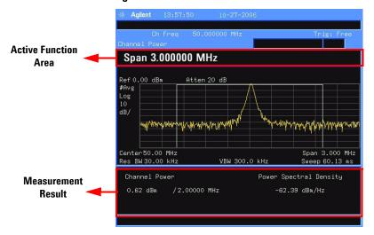
Figure 28 Channel Power Measurement
