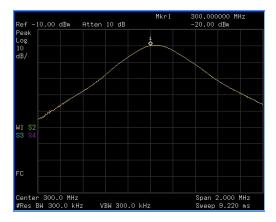
4 Change the resolution bandwidth (RBW) to 100 kHz so that the RBW setting is less than or equal to the frequency separation of the two signals:
