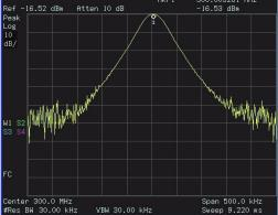
**5** Reduce the resolution bandwidth filter to view the smaller hidden signal. Place a delta marker on the smaller signal:
