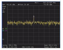
Note that increasing the attenuation moves the noise floor closer to the signal level.
