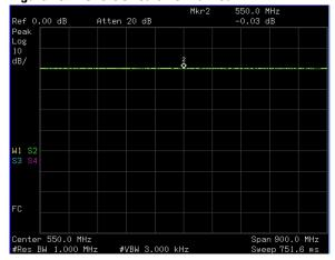
Figure 23 Short Circuit Normalized
