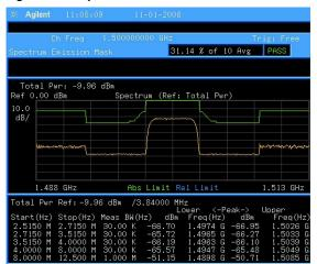
Figure 32 Spectrum Emission Mask
