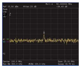
Figure 3 Delta Marker with Reference Signal Off-Screen
