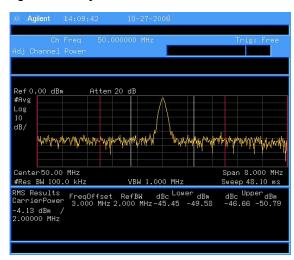
Figure 30 Adjacent Channel Power Measurement
