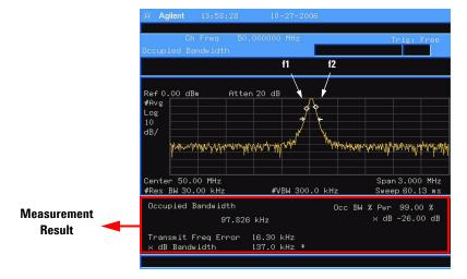
Figure 29 Occupied Bandwidth Measurement
