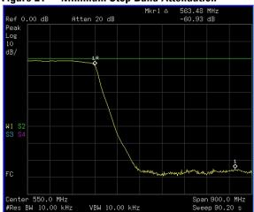
Figure 21 Minimum Stop Band Attenuation
