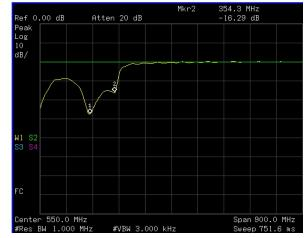
Figure 24 Measuring the Return Loss of the Filter
