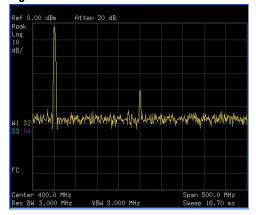
The signal produces harmonic distortion products (spaced 200 MHz from the original 200 MHz signal) in the analyzer input mixer as shown in Figure 16.
