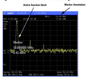
2 Use the knob, the arrow keys, or the softkeys in the **Peak Search** menu to move the marker. The marker information will display in the upper-right corner of the screen.
