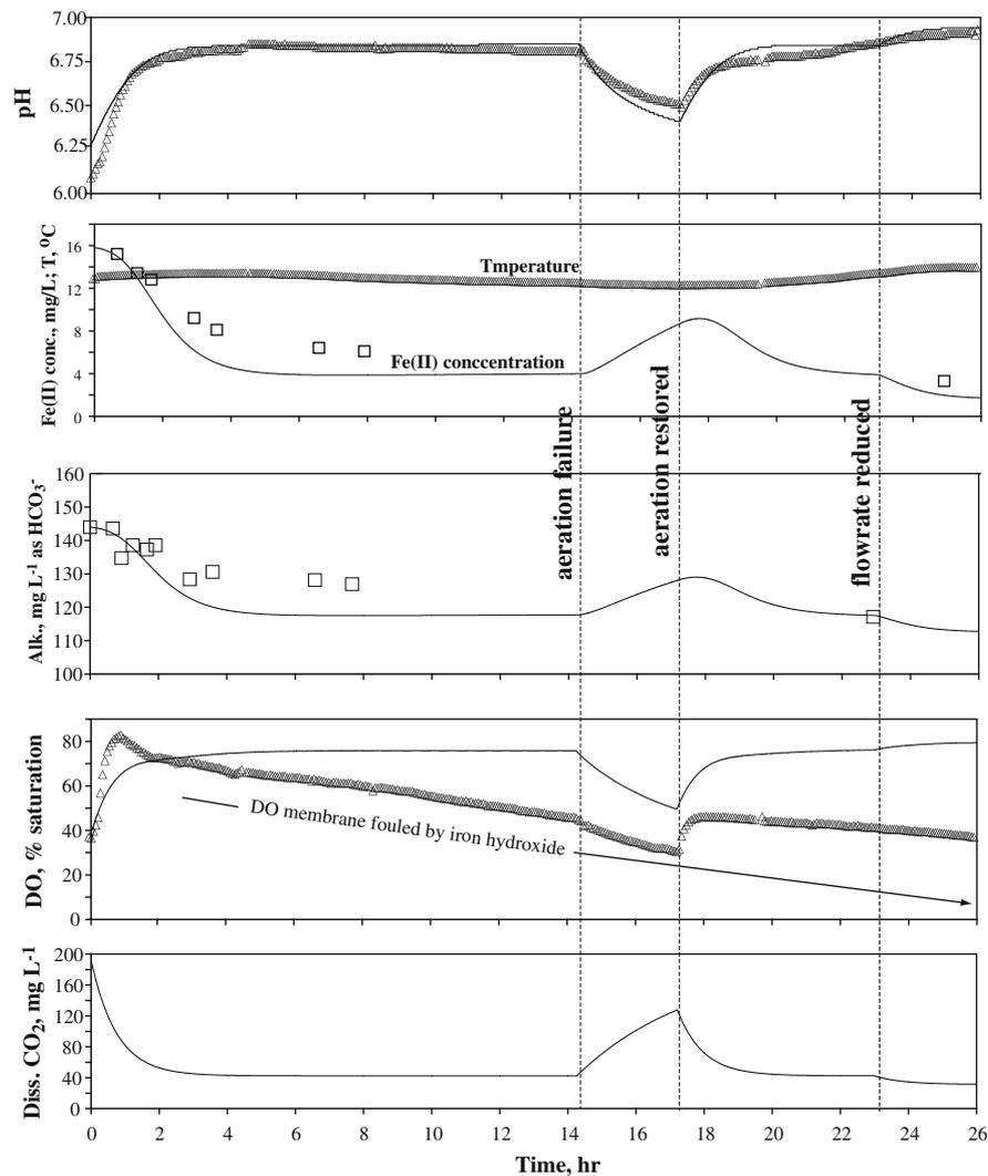
Fig. 6. Measured data (symbols) and Model 2 results (solid curves) for pilot-scale Site 21 aeration experiment.
