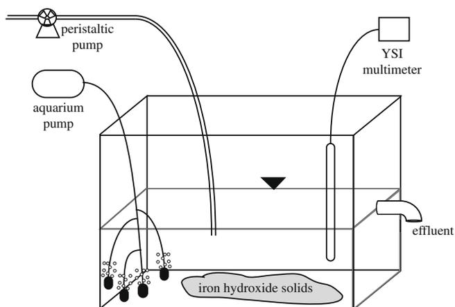
Fig. 1. Schematic diagram of 14-L flow-through reactor.
