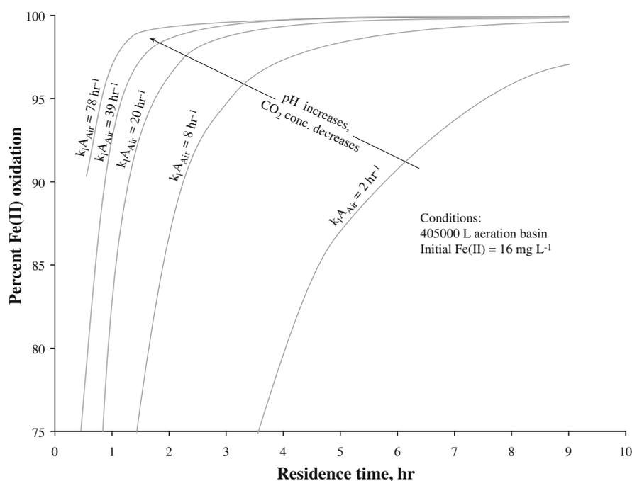
Fig. 7. Model 2 results for % Fe oxidation versus residence time for a full-scale treatment of Site 21, contoured for different mass transfer coefficients ( $k_l A_{Air}$ , governed by aeration effectiveness).
