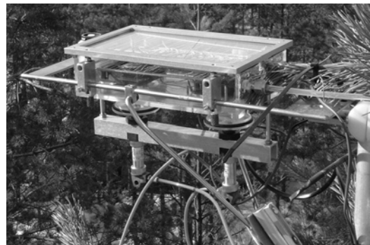
Measuring carbon dioxide uptake rates of trees (here by a branch cuvette in Hyyttiälä / Finland).
